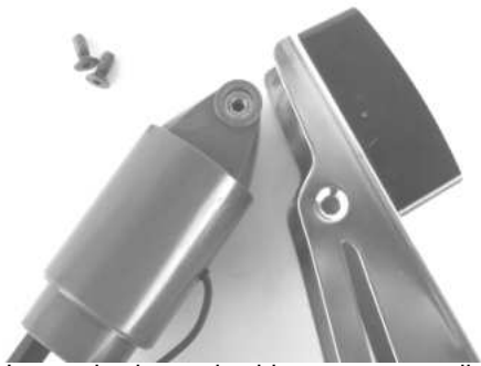
19. Insert the brass bushing remove earlier and secure with the original screws.
