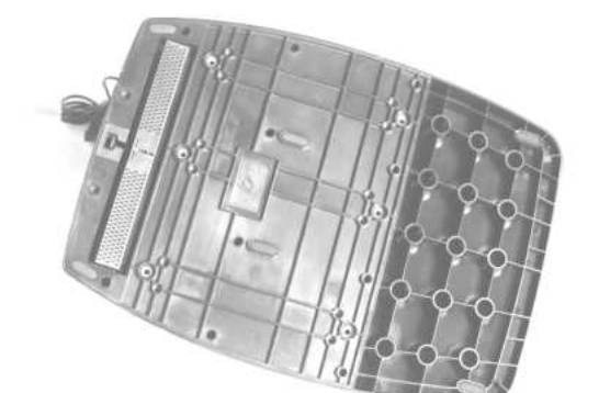
26. Place the bottom cover back on the housing and be sure it drops into place evenly all the way around.
