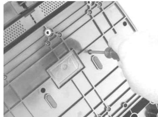
28. Secure the cover using the original 14 silver screws and 12 black screws removed at the beginning of the installation. Don't forget that 2 screws go under the carpet gripper.
