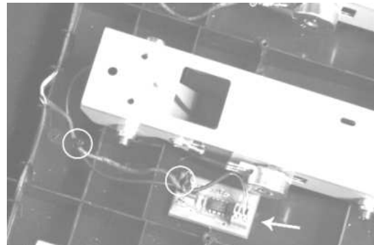
24. Using the remaining wire ties, strap the load cell wire to the original pedal wiring as indicated by the circles above. Peel off the backing on the mounting pad on the back of the interface board and secure to the plastic base as shown.
