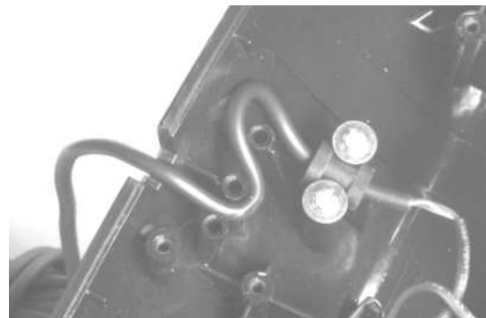
25. Make sure the cable exiting the housing is routed properly through the posts.
