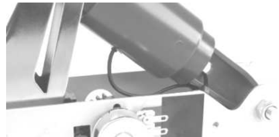
20. Insure the wire is kept away from the moving parts in the pedal assembly.
