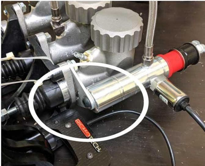
The brake pedal has been secured in the down position to prevent air from getting trapped at the pressure sensor during shipping. This is done to avoid the need to bleed the brake at the time of installation. Do not remove the strap yet.
