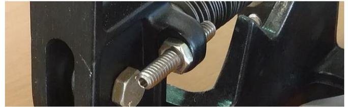
When any adjustments are made to the travel of the throttle or clutch pedal, those pedals should be recalibrated by setting the new Absolute Min and Absolute Max in the SmartPanel software.
