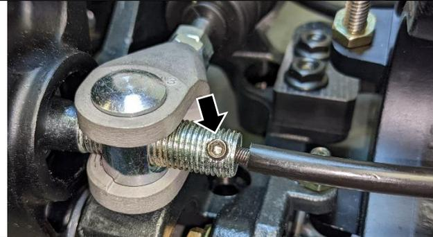
If the balance bar has a hole on the end and a set screw (arrow) then insert the end of the cable as shown and secure with the set screw.
