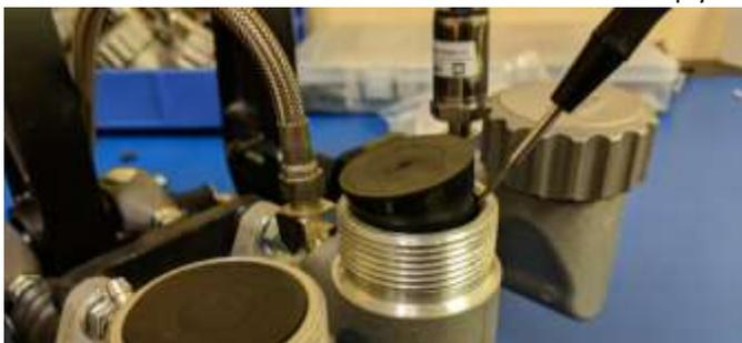
Remove the "leak-prevention" stoppers from the reservoir
