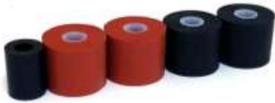
An optional brake tuning kit is available for those that want to tailor the sensation of the brake pedal. The kit includes two soft bushings (orange), two medium bushings (black), and one hard spacer. When these are used in conjunction with the original bushings (hard red bushing and extra-hard black bushing) there are 10 combinations possible.
