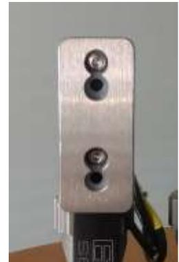
and 3 different positions horizontally. The height can be adjusted to two different positions by moving the pedal face to the other screw hole and can be set to 2 additional positions by flipping the pedal face upside-down.
