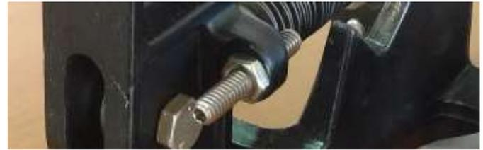
When any adjustments are made to the travel of the throttle or clutch pedal, those pedals should be recalibrated, as per Step 5, in the PCU box so the electronics learns the new range of travel for the pedal.
