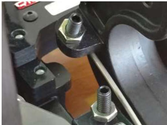
Similarly, the clutch pedal ending position can be adjusted by turning the stop screw located to the right of the pedal. Turning the screw clockwise will reduce the travel, while turning the screw counter-clockwise will increase the travel. Tighten the jam nut when the adjustments are complete to prevent the setting from changing.
