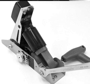
8. Remove the brake pedal assembly from the housing. Using a 10mm wrench and a 5mm Allen Key, remove the pivot from the base that secures the lower telescoping spring housing.
