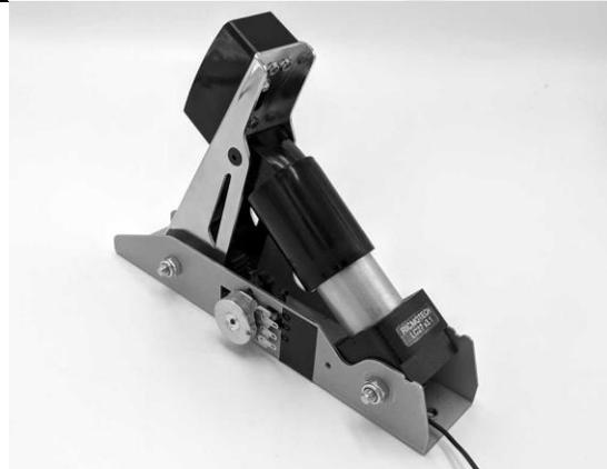
11. Compress the spring to align the square cutout in the load cell housing with the pivot hole in the base and insert the pivot pin. Secure the pivot pin with the 10mm nut.
