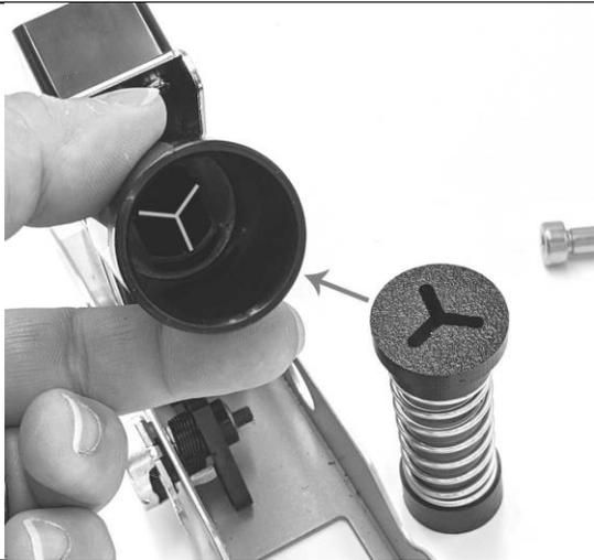
9. The upper spring housing has a 3-spoke blade inside. This is obstructed by a white cap on the G28 and G920 pedals. Remove the white cap to expose the 3 spokes. The spring assembly has the mating slot to fit around them.
