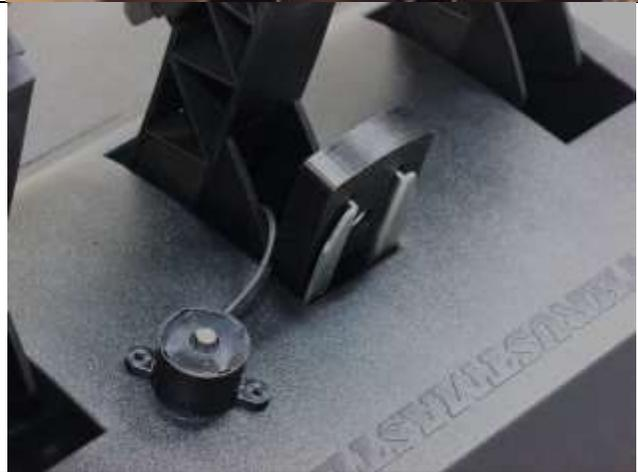
Pull the excess wire through the pedal and install the bracket and adapter assembled earlier as shown. Mount the bracket using the original screw and position. Verify the wire is not pinched by wiggling it at one end and verifying it wiggles freely at the other end.
