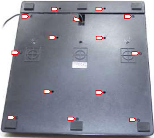
Remove the 14 screws from the bottom cover of the pedals. Do not overlook the screw behind the wire.
