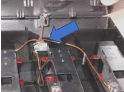
Place the cover back on the pedals as shown and reach in to plug the 6-pin connector back into the circuit board.
