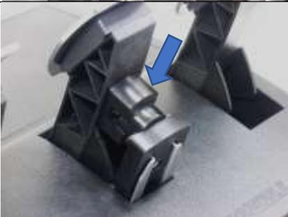
Mate the load cell and bushing housing with the bushing pressing against the metal tip of the load cell module. Slide the components between the back of the brake pedal and the adapter bracket as shown. Slide down until the holes on the load cell align with the holes on the adapter bracket.
