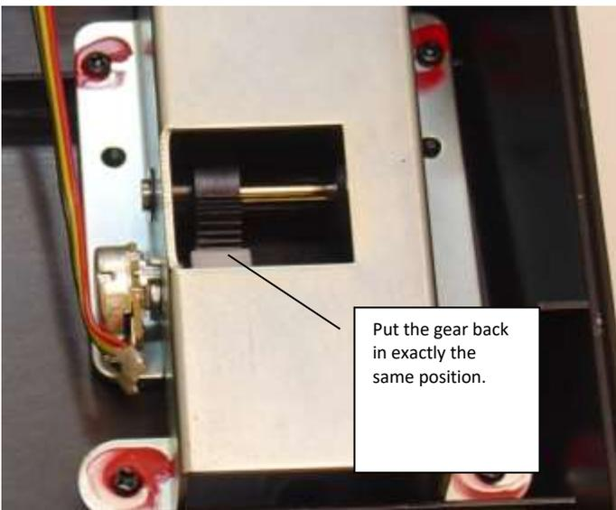
6. Place the pedal back into position and ensure the gear goes back the same way it was.
