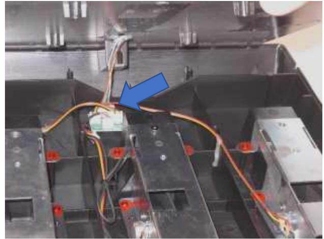
8. Place the cover back on the pedals as shown and reach in to plug the 6-pin connector back into the circuit board.
