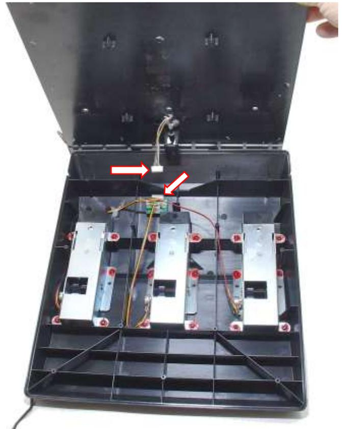
2. Carefully lift the cover from the near end with one hand and reach in with the other hand to disconnect the 6-pin plug from the circuit board. Do not lift the cover abruptly as this may cause damage to the connector. Set the cover aside.
