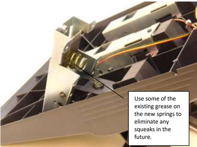
5. Being careful not to damage the wire, lift the pedal housing enough to reach the spring. Remove the original spring and smear some of the grease onto the ends of the new spring.
