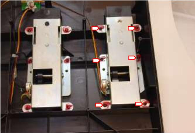
4. Perform the installation of the spring on one pedal at a time. Remove the six (6) screws holding each pedal in place.
