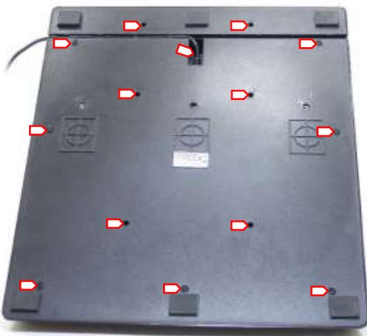
1. Remove the 14 screws from the bottom cover of the pedals. Do not overlook the screw behind the wire.
