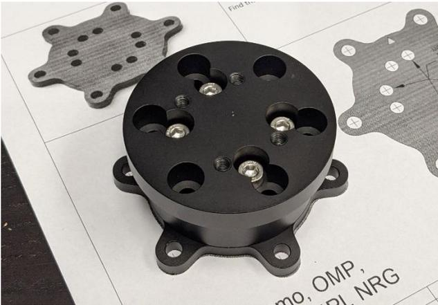
Use the 4 long screws and washers from the previous step to secure the spacer to the star plate as shown.
