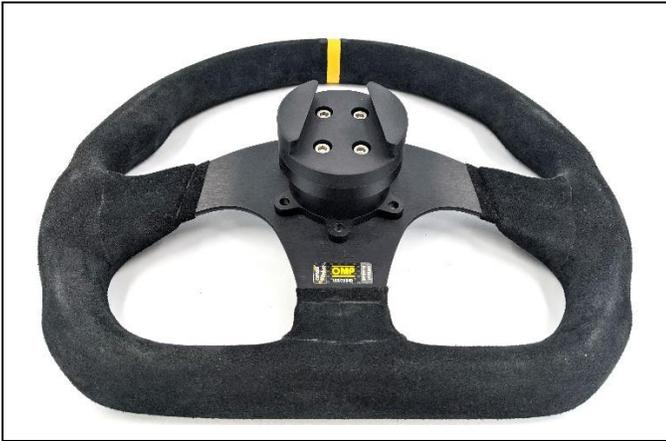
Orient the assembled quick release on the back of your steering wheel. Orient the quick release with the narrow part of the wedge to the 12 o'clock position.
