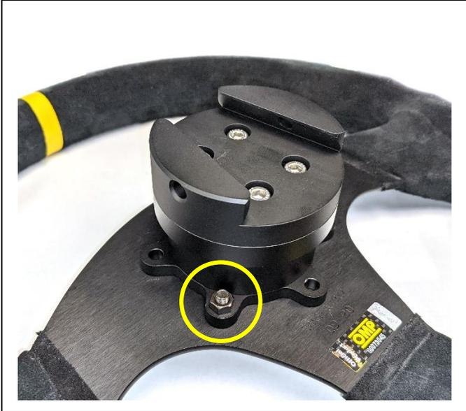
Using appropriate M5 screws and nuts (not included), secure the assembled quick release to the back of your wheel.
